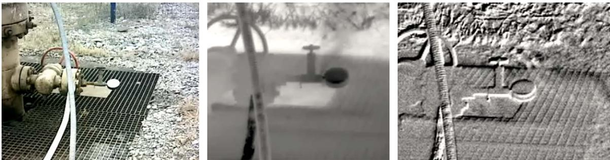
Fig. 11: leak detection and quantification using a FLIR camera (location 229, 6 October 2019)
