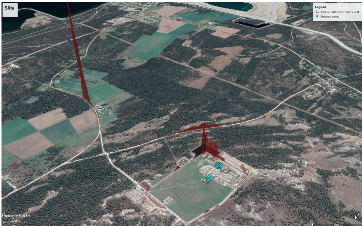
Figure 6.4. Relative atmospheric methane concentrations recorded when following the road around Slite landfill and on the road just downwind. Background methane concentration is subtracted and the maximum
