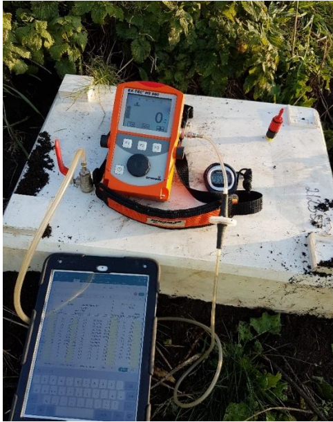
Figure 3.7. Flux chamber measurement set-up. Photo: Sweco Environment.
