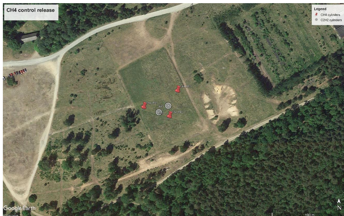
Figure 5.1. The tracer gas configurations in methane controlled release campaign. Red pins mark the methane release. The location of the tracer gas releases are marked with white circles.
