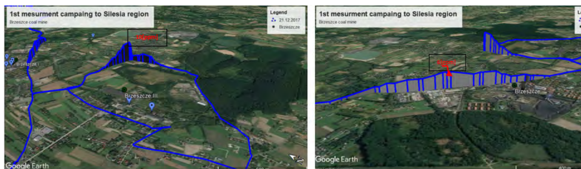
Fig. 6.3.4: Google Earth plot of methane plume elevation; left: Brzeszcze III mine shaft; right: Brzeszcze V mine shaft
