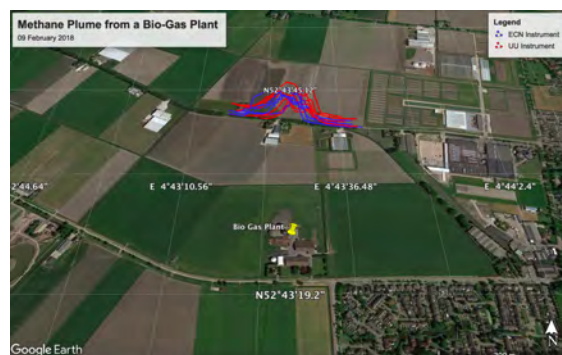
Fig. 6.10.5: Methane Elevations emitted from the biogas plant (yellow pin); measured by ECN (blue) and UU (red) instruments
