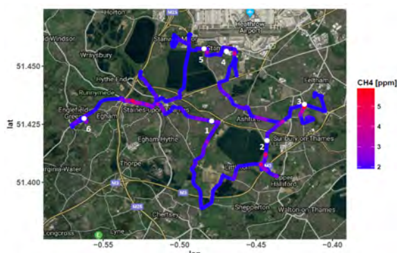
Fig. 2.13: Map of CH 4 concentration measured during urban area survey, 27.06.2018, white points and number indicate stops for changing to replay mode
