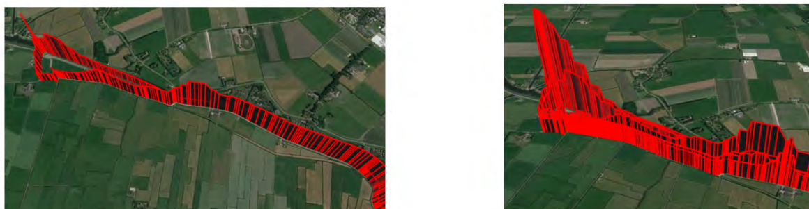
Fig. 6.3.7: Identification of methane plume, the left figure represents all measurement day- release test and data from 2 farms. The right figure represent only data obtained during release test – without values obtained from farms.
