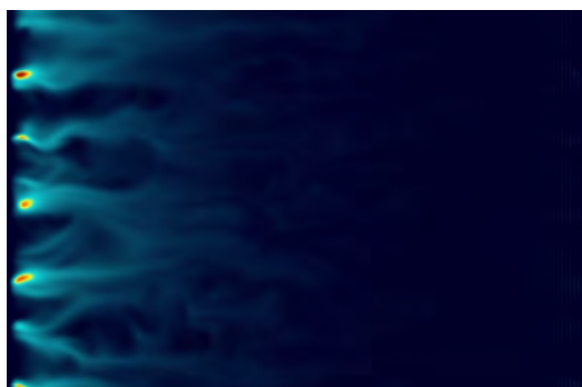
Fig. 2.20: DNS simulation of a plume from a line source in stationary homogeneous turbulence.
