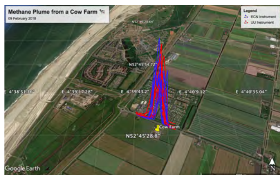
Fig. 6.10.4: Methane Elevations emitted from Lefjeshoeve farm (yellow pin); measured by ECN (blue) and UU (red) instruments
