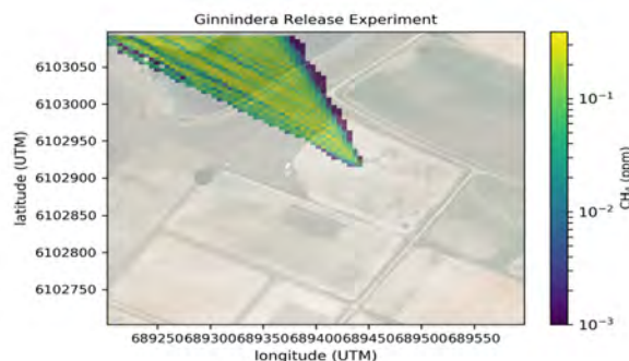
Fig. 8: Simulated Methane mixing ratio field from the Tracer release experiment performed in Ginnindera, Australia using GRAL model. Sampling height was taken at 2 m above ground, which is also the same height at which the outlet of the methane bottle is located.
