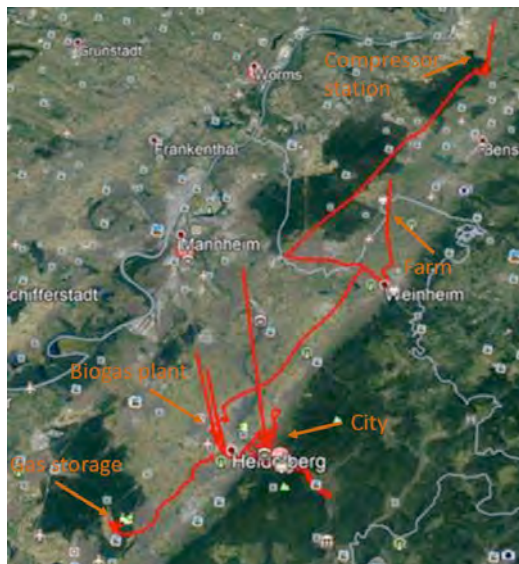
Fig. 2.1: Typical transect of 6 hours of measurement in Heidelberg and surroundings with concentration peaks at a biogas plant, in the city of Heidelberg, close to a farm and a natural gas compressor station
