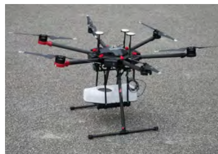
Fig. 6.6.4: DJI Matrice 600 drone equipped with the methane sensor
