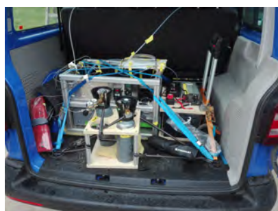
Fig. 6.1.1: Mobile CRDS analyser in vehicle.
