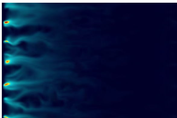
Fig. 6.11.3: DNS simulation of a plume from a line source in stationary homogeneous turbulence, following the simulation by Moser et al. (1999)
