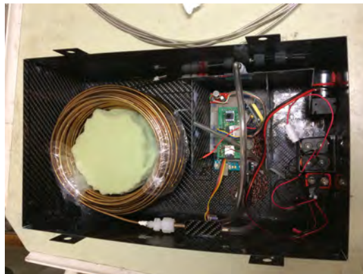
Fig. 2.4: a) a schematic design of the UAV AirCore system, b) an image of the UAV AirCore system
