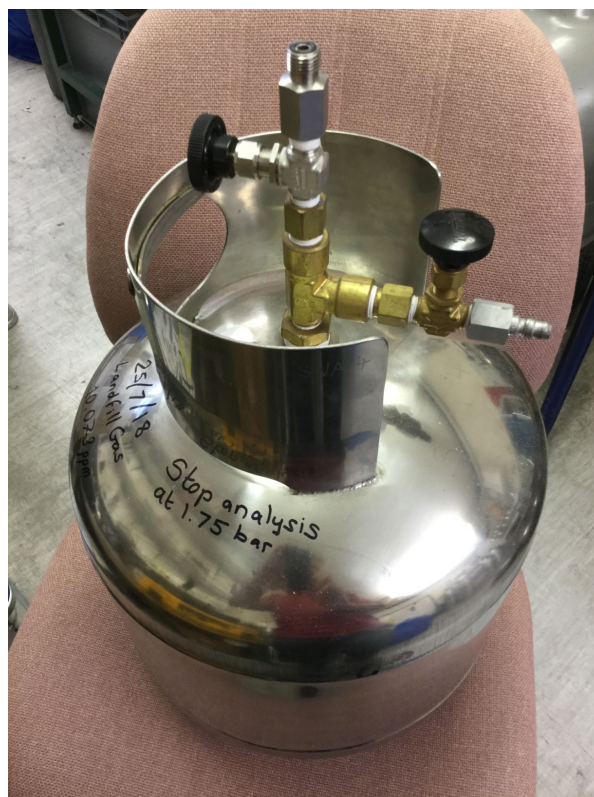
Fig. 1: One of the stainless steel flasks sent to UU for inter-comparison measurement
